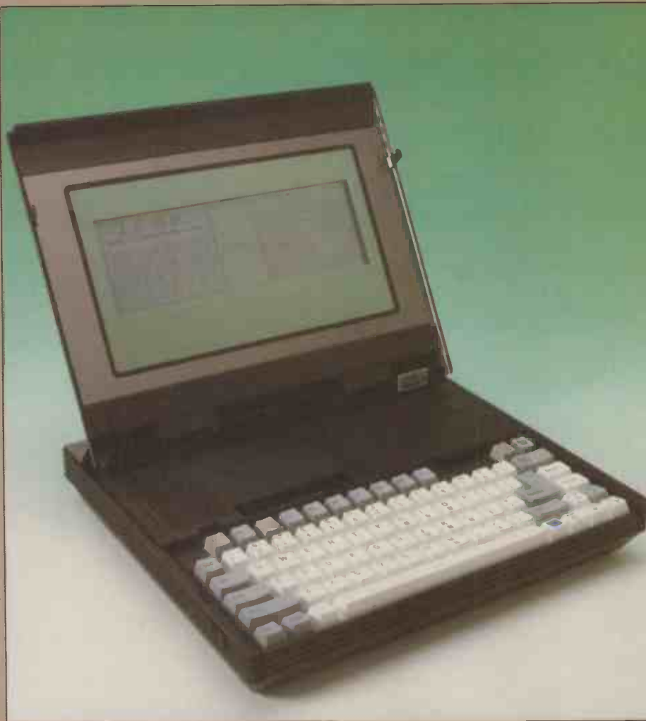
The detached keyboard is unusual for a lap portable, but it helps when placing the LCD screen for the best viewing positions.
